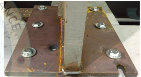
Figure 3.2: Mounting Detail
