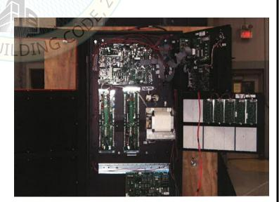
UUT1 was wall mounted - rigid using four (4) 1/2" bolts and washers.
