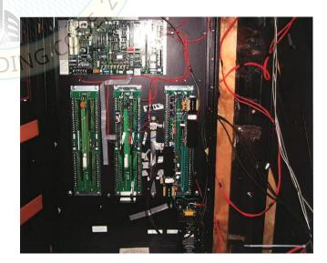
UUT2 was wall mounted - rigid using four (4) 1/2" bolts and washers.
