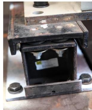
UUT7 was mounted on a test fixture (total wt. 3,815 lbs.) that was base mounted - rigid on four (4) VMC MSSH-1E-1000 which were locked to simulate rigid mounting. The isolators were fastened to the table using four (4) 5/8" SAE Grade 8 bolts, washers and one (1) 3/4" SAE Grade 8 bolt each to fasten the UUT to the isolators.
