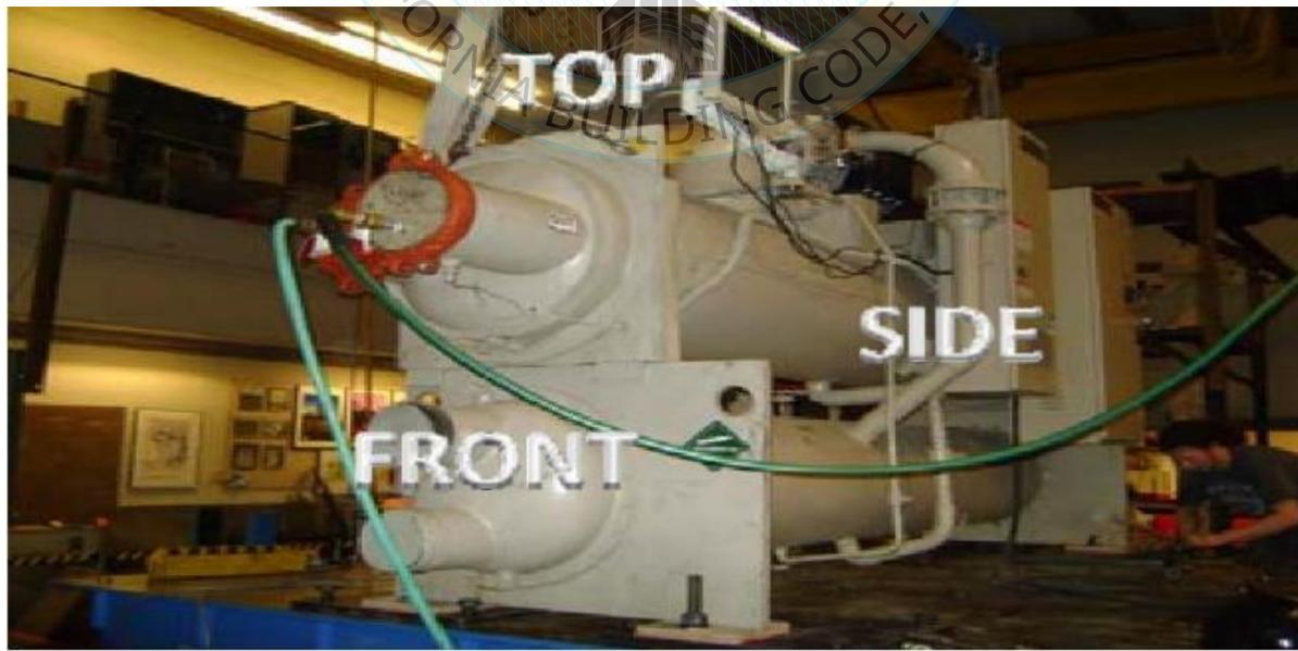
UUT1 was base mounted - isolated in 1/4" neoprene pads with eight (8) 1" Grade 8 bolts.
