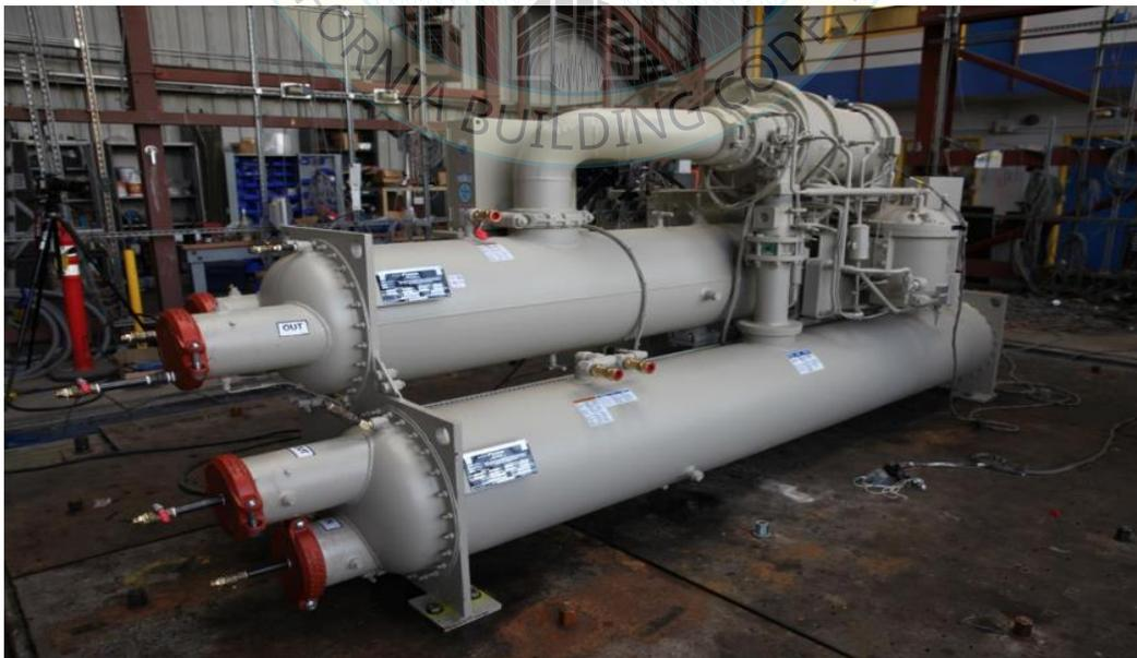
UUT5 was base mounted - rigid to the table using eight (8) 1" SAE Grade 8 bolts and washers.
