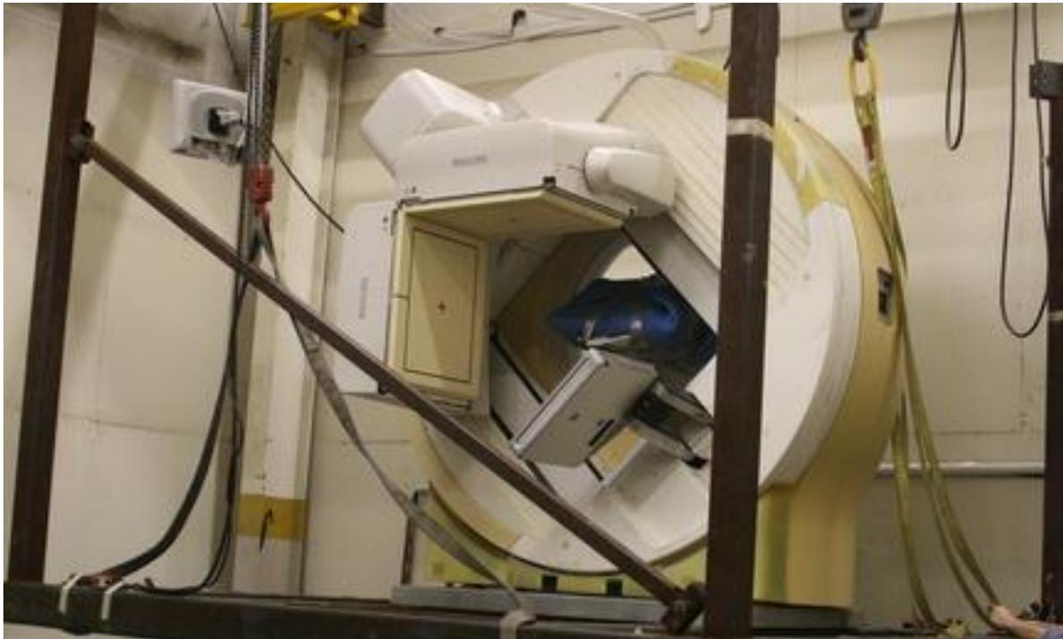
**Figure 12: Brightview XCT Gantry Test Mounting**
