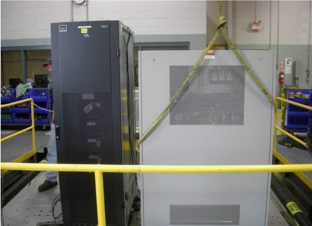
Figure 1: NX Bypass Distribution Cabinet (left) and PPC 200kVA UPS (right)
