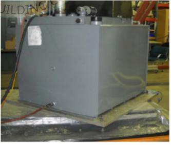
Component maintained structural entegrity and functionality after shake table tests. Rigid base mounted to the test table fixture using (6) 3/8" diameter SAE Grade 8 bolts.
