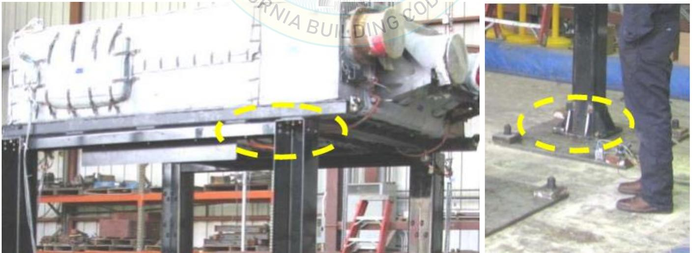
CEM rigid base mounted to frame with (16) 3/4" A490 bolts. Frame rigid mounted to fixture plates with (16) 7/8" A490 bolts. Unit maintained structural integrity and remained functional per manufacturer requirement after shake table test. Contents were included in testing per operating conditions.
