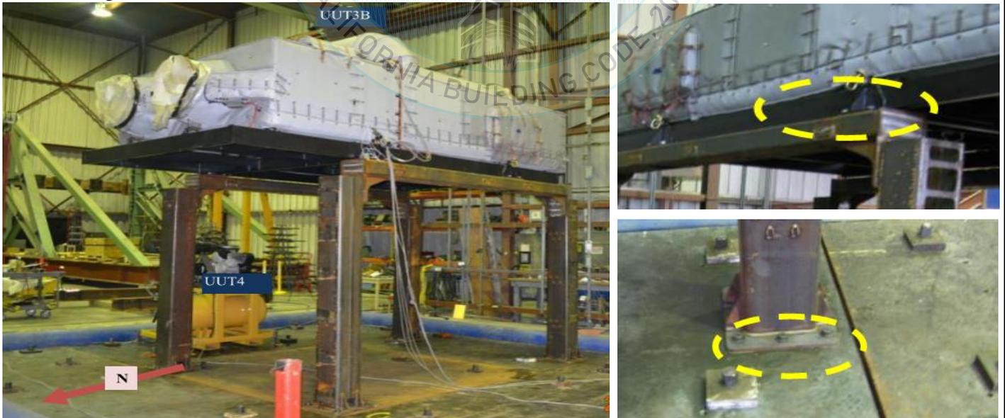
CEM rigid base mounted to frame with (16) 7/8" Grade 8 bolts. Frame rigid mounted to fixture plates with (24) 3/4" Grade 8 bolts. Unit maintained structural integrity and remained functional per manufacturer requirement after shake table test. Contents were included in testing per operating conditions.
