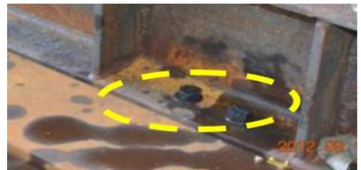
CEM rigid base mounted to beams with (16) 7/8" Grade 8 bolts. Beams rigid mounted to fixture plates with (8) 3/4" Grade 8 bolts. Unit maintained structural integrity and remained functional per manufacturer requirement after shake table test. Contents were included in testing per operating conditions.
