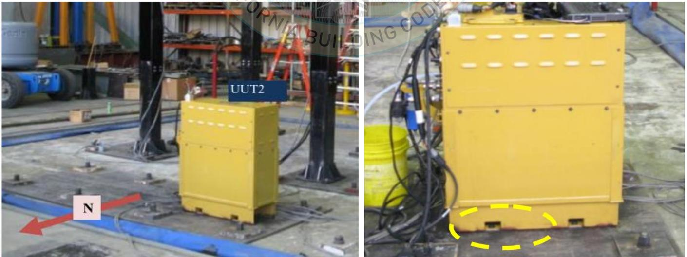
Rigid base mounted to fixture plate with (8) 3/8" A490 bolts.
