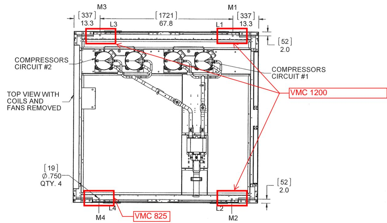
BLANK PANELS ARE USED ON UNIT SIDES. SLOPED 50° COILS USED ON INSIDE.
