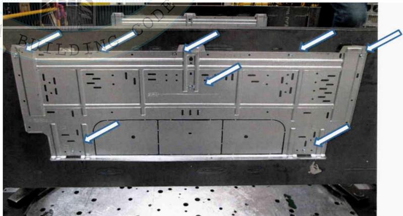
Wall mount plate was fastened to wall fixture using eight (8) #10 self-tapping screws. UUT hangs on the wall mount plate and snaps into the wall mount plate.
